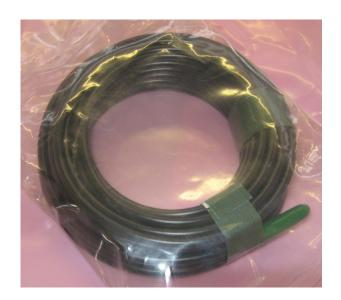
Safety Fuze is used in demolition work where a delay is required to give personnel time to retire to a place of safety before the charge detonates.
